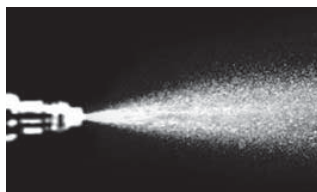
Injector spray pattern after P.i. treatment.
